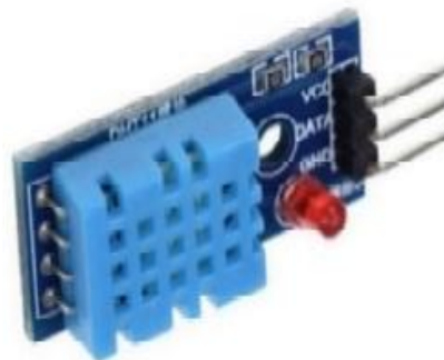
Figure.4: Digital Humidity and Temperature sensor module
